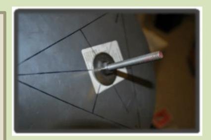
2) Thread 2 hex nuts onto the threaded rod. Thread one nut 15 inches from the end. Thread another one 3 inches from the same end.
