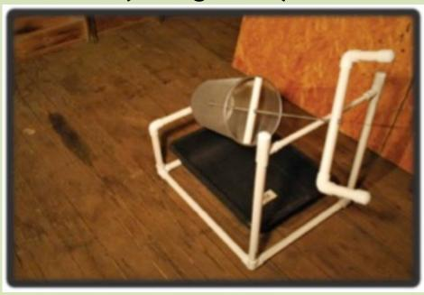
The Urban Worm Castings Harvester accommodates a small concrete/mortar mixing tub to catch the castings, though a shallow Sterilite or Rubbermaid bin would work fine too. Though the trommel can be rotated manually, it can also be rotated using a power drill on low speed by affixing a 5/16-in socket attachment (check size) to a bit driver. This is my preferred option.
